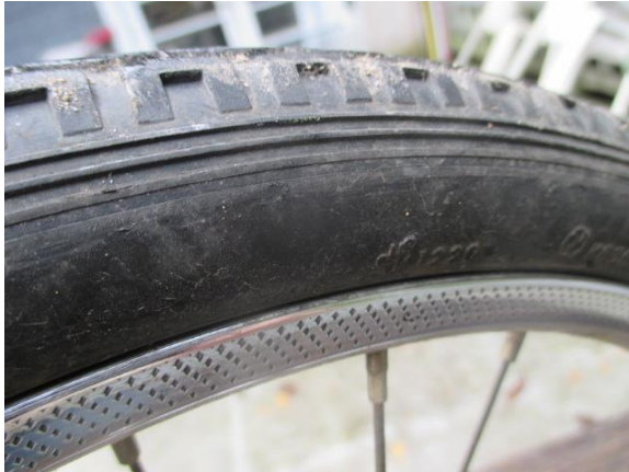
Sipes on rim of 20" Victoria folder, for wet braking
