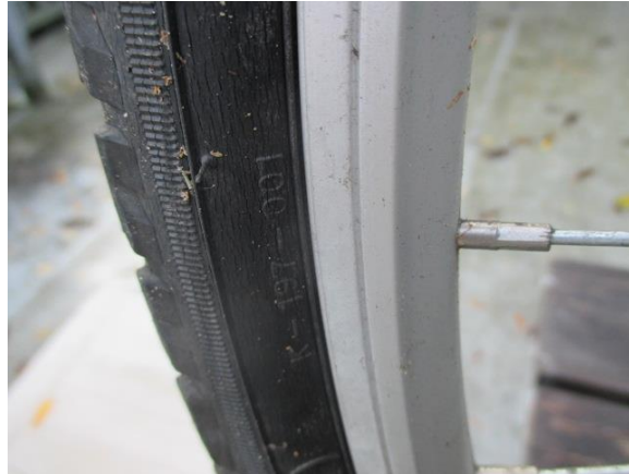
Condemning groove on aluminium rim of Asama Euro7
